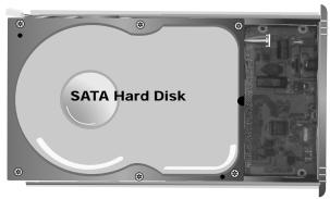
5) Locate the screws included in the package. Ensure that the screw guides on the bottom of the HDD are aligned with the openings on the bottom of the drive tray. Fasten the HDD to the drive tray by inserting and tightening the screws.
