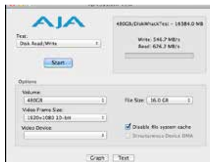
此读取与写入速度的测试环境: MacBook Pro 8.3, Mac OS X 10.7.3 (Disk Utility), Intel 520 Series 240GB SSD, RAID 0.
